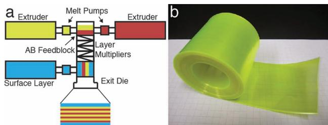
**Figure 1.** (a) Schematic of the co-extruder used to manufacture the films, and (b) the resulting roll of films. The neat polymer and polymer/dye blend are loaded into the extruders, melted, and pumped through the two-layer feedblock, and then into a series of layer multiplication dies, each of which doubles the number of entering layers. A final extruder adds surface layers for mechanical stability. The film in (b) is 6 cm wide and on the order of 100 m long.
