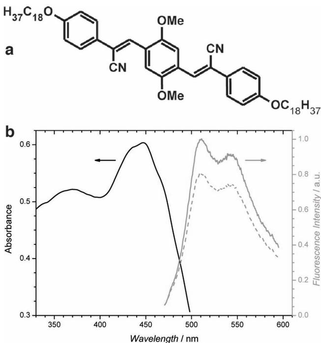
**Figure 2.** (a) Chemical structure of the dye (C18-RG). (b) Absorption (black) of the entire 200  $\mu\text{m}$  thick ML film, containing 64 active layers, and the FL spectra of a single layer before (grey) and after (dashed) writing indicating a typical level of FL reduction induced by writing.
