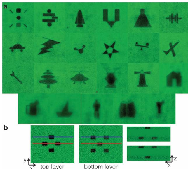
**Figure 3.** (a) Patterned images stored in the 23 layer film (false color). Top left is the topmost layer and bottom right is the lowest layer, with subsequent layers going from left to right. (b) Cross-section of two layers after writing complementary images. The top cross-section is along the blue line, and the bottom along the red line. Images are normalized to the background. Each image is 22  $\mu\text{m}$  square, containing 512 pixels.
