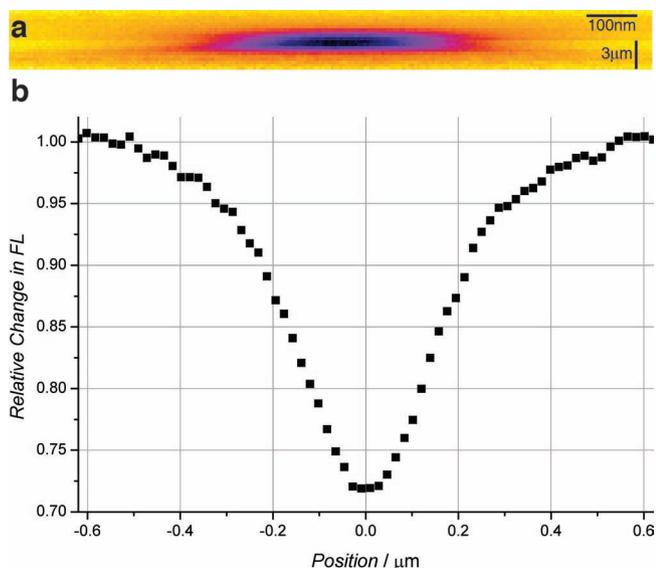
**Figure 4.** (a) Cross-section of a single written line in a 5 μm thick single active layer. The raw FL intensity was normalized by background and averaged over the length of the line. (b) Intensity profile of the spot at the waist, with a FWHM of 380 nm.
