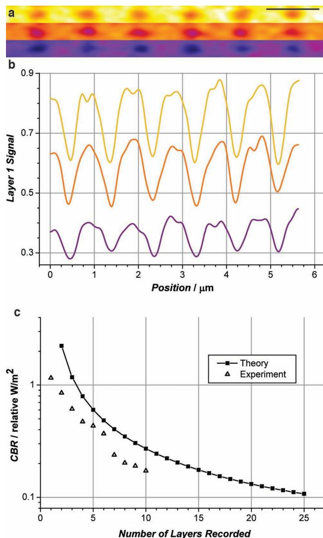
**Figure 5.** (a) FL images of a series bits in layer 1 after recording layer 1 itself (top), layers 1-5 (middle), and layers 1-10 (bottom). Images have the same brightness and contrast settings. Scale bar is 1 μm. The curves in (b) show the modulation signal of the images in (a). (c) The experimentally measured CBR of layer 1 versus the number of layers of recorded, along with results of simulation assuming a photobleaching process which is linear in optical fluence.
